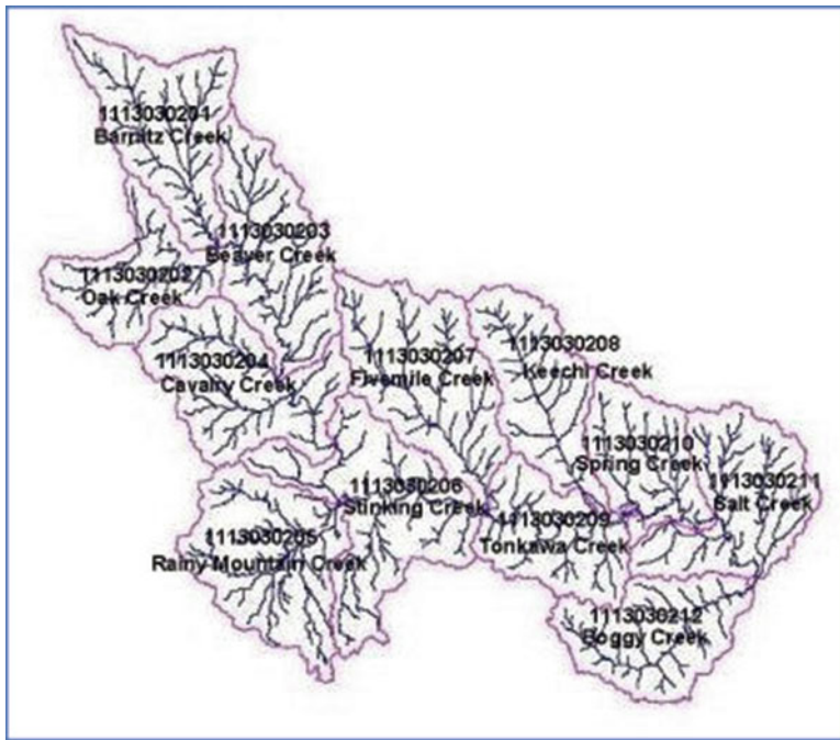
Fig. 7.9. Watersheds with Pfafstetter index numbering [20].
